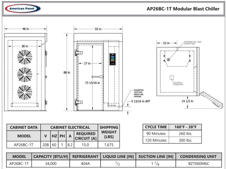
Note: Refrigeration shall be a medium temp. system (40°F to -10°F SST), rated @ 14°F SST, 105°F Cond.
