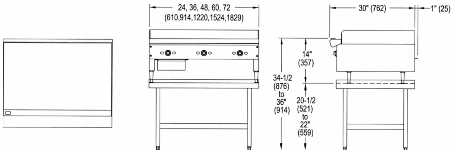
**HEAVY DUTY THERMOSTATIC GRIDDLES: Highly polished 3/4" thick plates**
