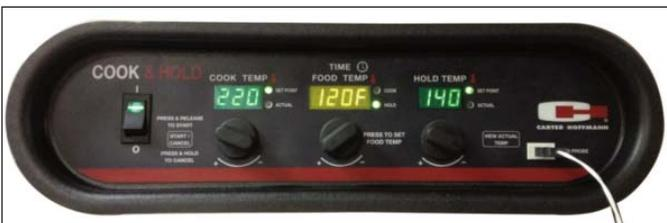
**EASY-TO-USE DIGITAL CONTROLS...** Control cooking and holding with separate dial controls and digital display. Cook according to time or according to product temperature with meat probe. Temperature range of 100°F to 200°F for hold cycle and 100°F to 325°F for cook cycle. Eighteen hour timer counts down in cook cycle. When cook cycle is over, cabinet automatically switches to hold cycle and timer counts up. Displays in Fahrenheit or Celcius scale.
