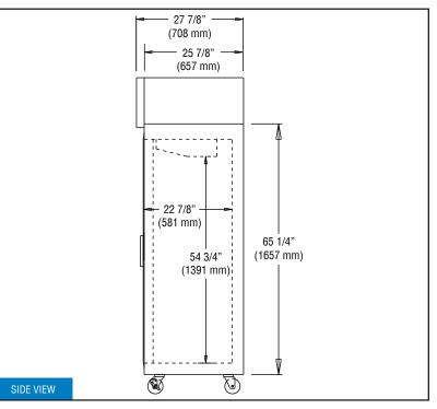
IMPORTANT NOTE: If the cabinet is located directly against a wall and/or under a low ceiling, a minimum clearance of 12" is required.
