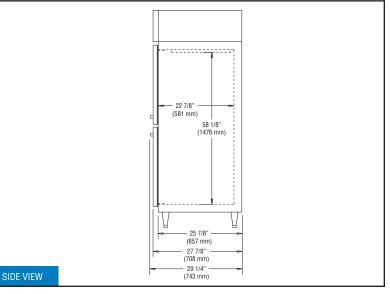
IMPORTANT NOTE: If the cabinet is located directly against a wall and/or under a low ceiling, a minimum clearance of 12" is required on top and 3" on sides and rear.
