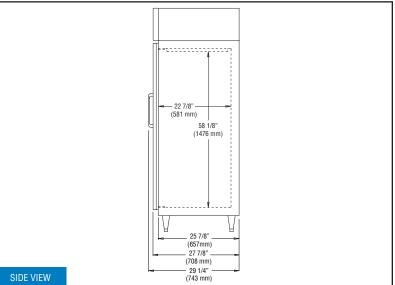
**IMPORTANT NOTE:** If the cabinet is located directly against a wall and/or under a low ceiling, a minimum clearance of 12" is required on top and 3" on sides and rear.
