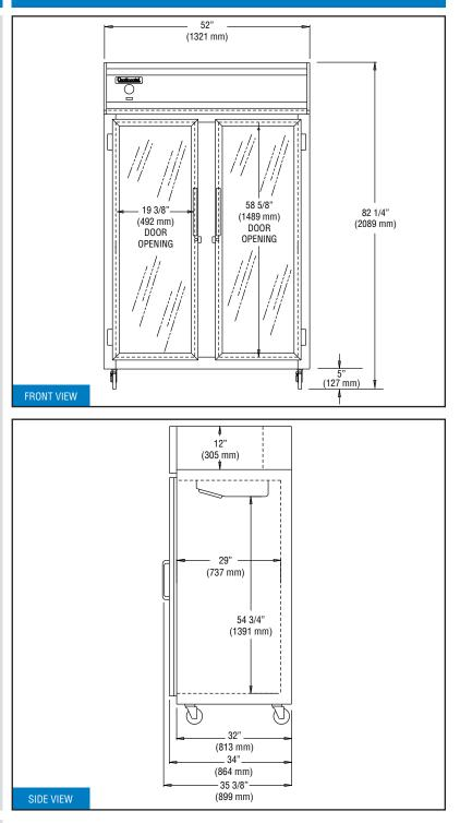
**IMPORTANT NOTE:** If the cabinet is located directly against a wall and/or under a low ceiling, a <u>minimum</u> clearance of 12" is required.
