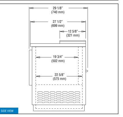
IMPORTANT NOTE: A minimum clearance of 3" is required on each side, front and rear of cabinet for optimum performance.
