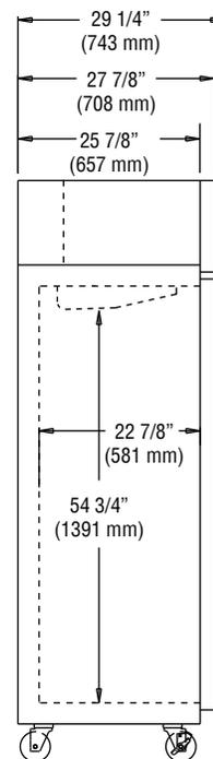
**IMPORTANT NOTE:** If the cabinet is located directly against a wall and/or under a low ceiling, a minimum clearance of 12" is required.
