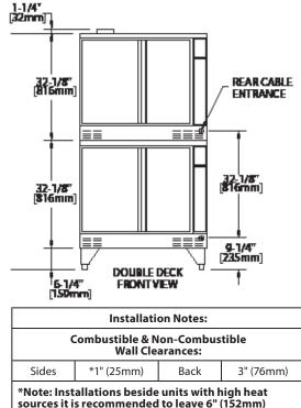
sources it is recommended to leave 6" (152mm) on the right side of oven. Refer to the installation manual for more detail
