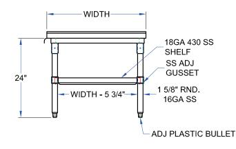
SOME UNITS SHIP UNASSEMBLED FOR REDUCED SHIPPING COST. ALL DIMENSIONS ARE TYPICAL. TOLERANCE +/- .500" John Boos & Co. is constantly engaged in a program of improving products and therefore reserves the right to change specifications without prior notice.
