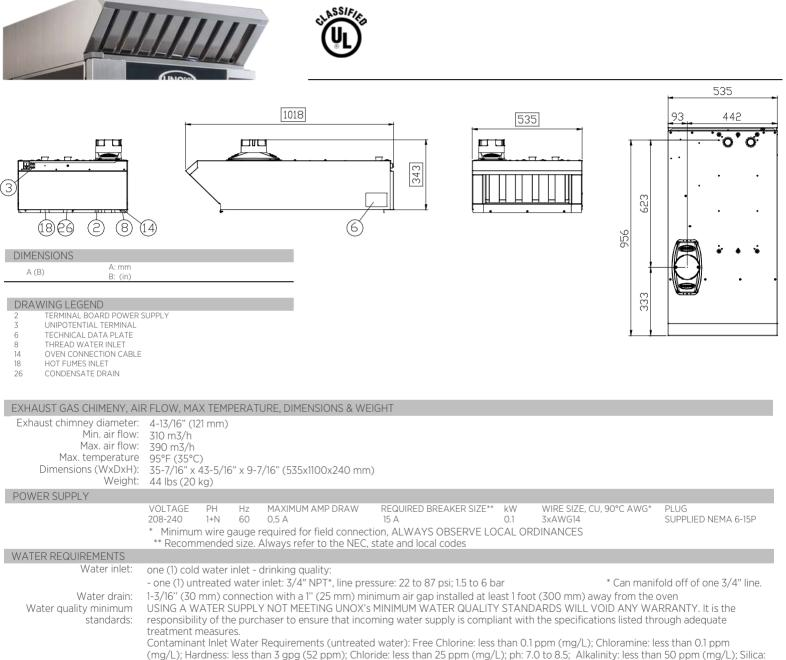
Oven must be installed level. Back-flow preventer integrated in the unit.
