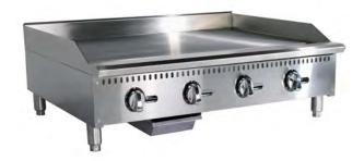
VALYR's heavy duty thermostatic gas griddles are designed to provide precise temperature control during your busiest hours. This 48-inch thermostatic griddle features a 3/4-inch thick smooth steel griddle plate that helps maintain consistent temperatures. Four manual burner controls allow for precise cooking temperatures along the cooking surface. Each "U" shaped stainless steel burner puts out 30.000 BTU/hr.
