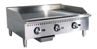
VALYR's heavy duty thermostatic gas griddles are designed to provide precise temperature control during your busiest hours. This 36-inch thermostatic griddle features a 3/4-inch thick smooth steel griddle plate that helps maintain consistent temperatures. Three manual burner controls allow for precise cooking temperatures along the cooking surface. Each "U" shaped stainless steel burner puts out 30,000 BTU/hr.
