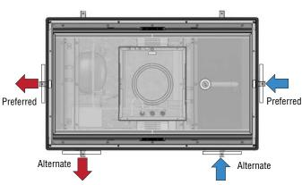
Customer supplied louvers must be installed in the surrounding cabinet to ensure adequate ventilation. One intake and one discharge louver are required. The preferred louver location is the short ends of the cabinet.
